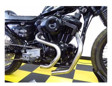
4. Install support bar racket onto the tab mounted on the exhaust. Leave it loose so you have plenty of adjustment range.
