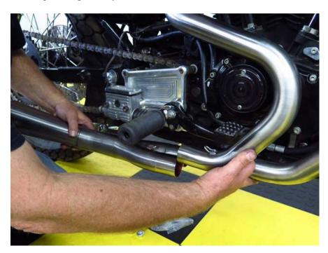
6. At this point you can decide whether you wish to use the provided sealant to help prevent collector leaks. Apply a light film to the inside of the collector inlets and to the outside of the header primary tubes. Let it dry just a little then slide them back together, cleaning up as you go.
