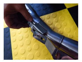
5. Slide the collector into place on the header tubes, *don't install springs yet*. (We normally recommend doing a complete dry fit first, then come back and install collector sealant).
