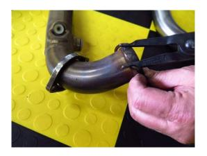
2. Check the gasket inside the cylinder head and also condition of the spring clips, replace if needed. Transfer the cylinder head spring clips and flanges to the new exhaust. Make sure the indentation in the flange (for the spring clip to sit in) is facing in the proper direction
