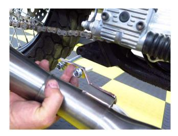
8. *Gradually* begin tightening up the entire system to reduce binding. Wiggling it here and there helps it settle in as you tighten it.
